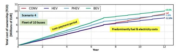
Figure 20. TCO time profile for different bus fleet types and Scenario 4 from Figure 18.
