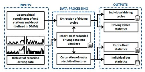
Figure 3. Flowchart of Data Post-Processing Module (DPPM).
