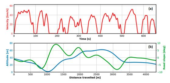
**Figure 4.** Sample of reconstructed driving cycle for city bus route Hotel Palace–Pile and afternoon hours: velocity vs. time profile (**a**) and road slope vs. distance travelled given along altitude source profile (**b**).
