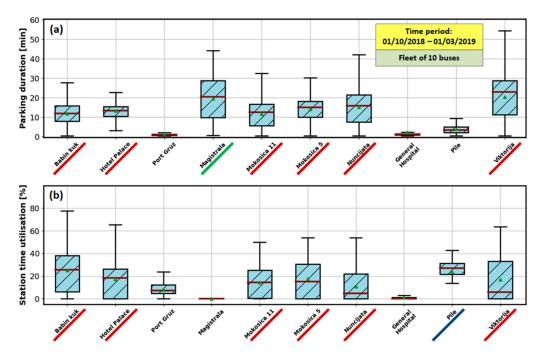
**Figure 7.** Boxplots of time duration of buses being parked at different end stations (**a**) and end stations charging utilisation (**b**).
