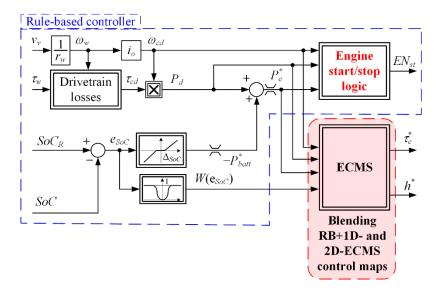
Figure 12. Block diagram map-based RB+ECMS control strategy.
