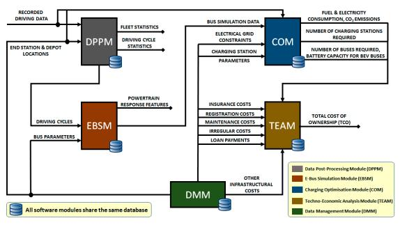
Figure 2. Organisational structure of simulation tool.
