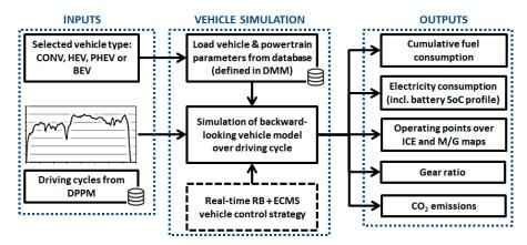
Figure 8. Flowchart of E-Bus Simulation Module (EBSM).
