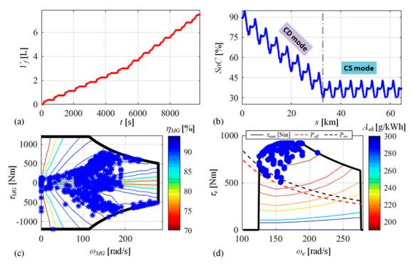
**Figure 10.** Simulation results for PHEV bus over the driving cycle given in Figure 4 repeated 15 times, including: cumulative fuel consumption time response (a), battery SoC vs. distance travelled (b), M/G machine operating points (c), and engine operating points (d).
